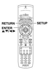
Then turn the jog dial or press the  $\blacktriangleleft$  or  $\triangleright$  cursor button on the remote controller to set the size of vour front speakers.
